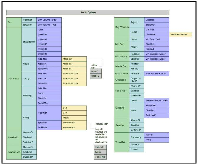
FIGURE 145. Audio Options Menu for the KP 32 CLD without GPIO Option card installed.
